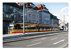
▲ A combined platform at Karlsruhe Durlach station with a height of 760mm for the Rhein-Neckar suburban railway (left) and 550mm for light rail (right).
