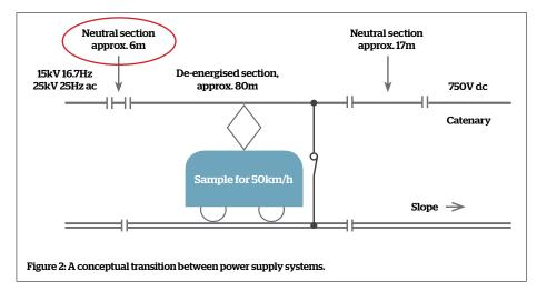
A conceptual transition design is shown in Figure 2 above. For reference, to the right we see such a transition in Karlsruhe, with the neutral section highlighted with a red circle.
