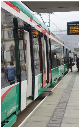
▲ Concept of low/medium-floor access points (front without and middle with moveable step) in Chemnitz. ➤
