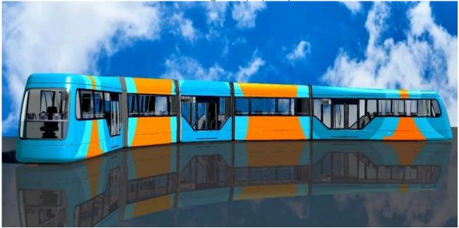
MRV-4 SERIES City Runner articulated multi-body trams is rated to carry 300 pax and can be coupled autonomously to a maximum two cars giving a maximum of 600 passenger
