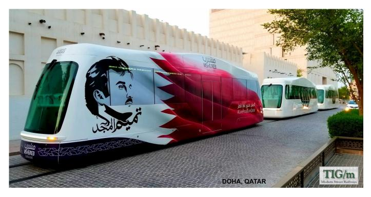
MRV-3 City Car single car body and is rated to carry 100 pax and can be coupled autonomously as above to a maximum of three as shown above and using suitable, safe sidings and unneeded car 2 or 3 can be parked off peaked eliminating unnecessary dead milage and wear and tear.
