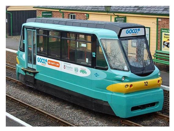
We offer services to communities that are seeking to promote and develop ultra light rail - that is, light rail with a basic and simple lightweight, affordable technology which gives a much lower cost to operate, lower costs per passenger Km than conventional light rail vehicles
