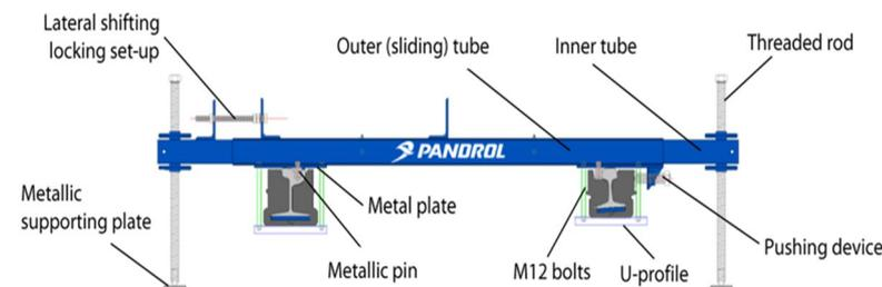
Typical Rail Positioning Jig
